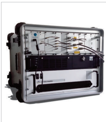
SpacEarth branded AIS-INGV ionosonde in a portable configuration complete with power amplifier and control PC.
