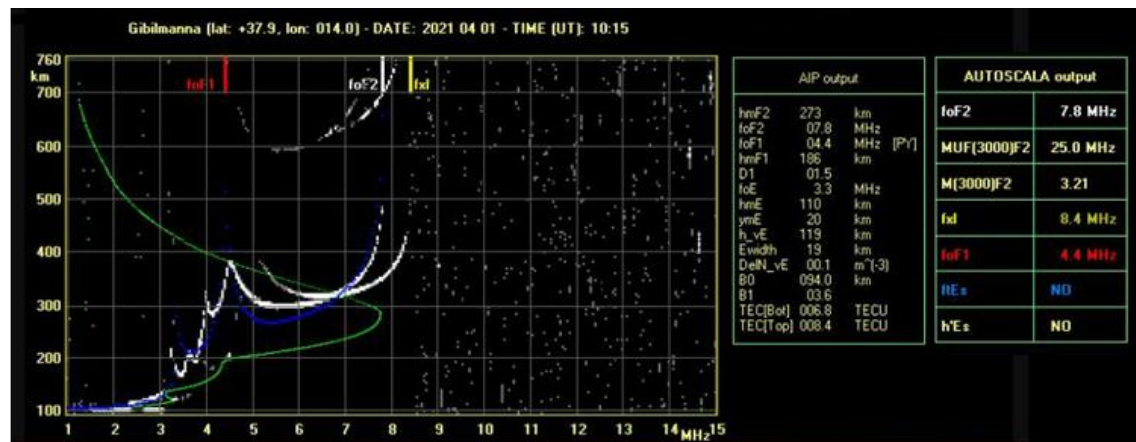
AIS-INGV ionogram with scaled parameters and profile
